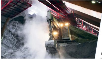
The bottom ash is washed with additional water in the slag extraction unit to reduce the content of readily soluble salts. It is sifted, broken up and freed from unburned components in order to produce a tested and approved building material comparable to a mineral mixture made from processed building rubble. The unburned components of the bottom ash are returned to the waste bunker to pass through the incineration process once more.
